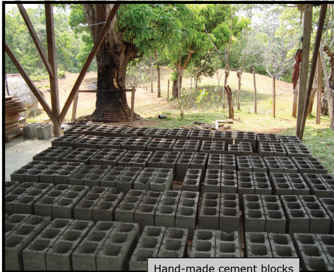
Hand-made cement blocks
